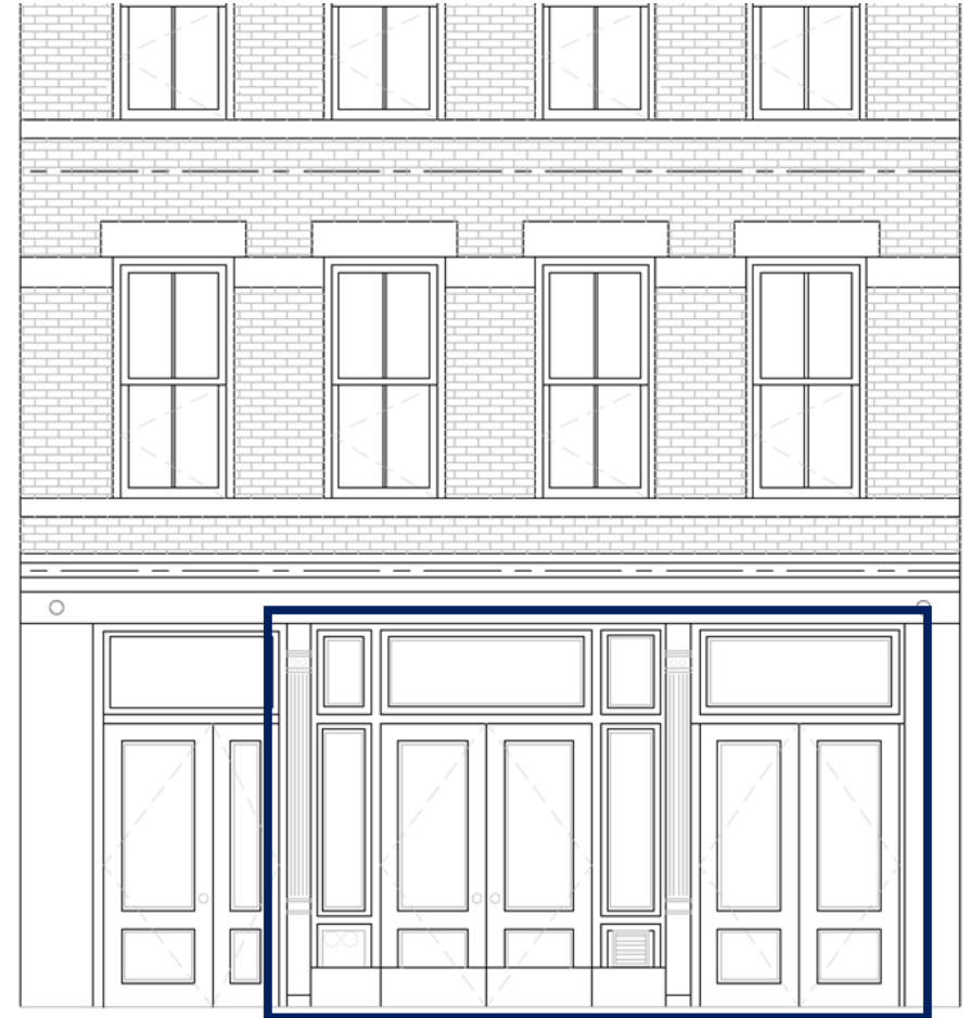
New storefront to be installed
